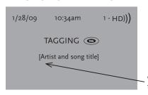
When the TAG button is selected, the broadcasted information will be saved and transferred to the iPod.
